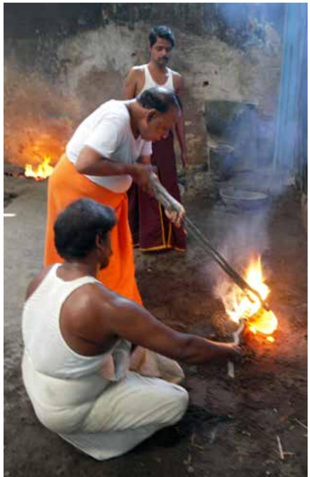
Pouring the bronze into the mould. The man kneeling down is holding a stick with a piece of sacking wrapped round the end and is holding back any dross on the top of the molten metal
