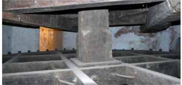
**Part of the gearing of the boring machine - the floor to the capstan is above and this drives the main gear wheel below**
