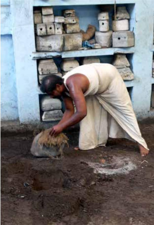
Once the mould is baked and hot and the wax has run out it is carried to the casting floor where a small depression has been made for it
