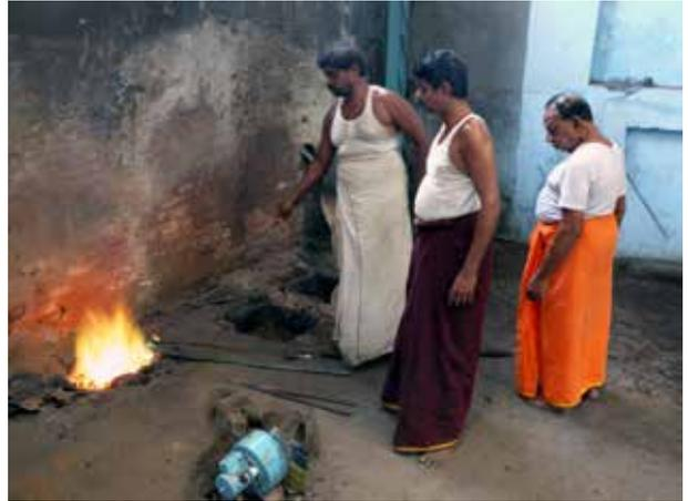
A small crucible of bronze is being heated up - air is pumped into the fire by the small electric fan in the foreground
