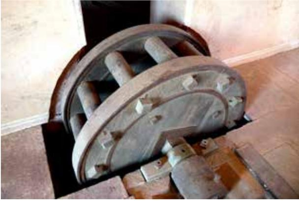
The final and fourth gear wheel - it is driven by a third gear beneath the floor which was impossible to photograph. The wall has been cut back to accommodate the wheel leading us to think that there has been some adaption or change to the original configuration. The 'chuck' to hold the boring bar is mounted directly in front. The gear, like the second and third gears, runs on copper alloy bearings, one of which can be seen here between the gear and the 'chuck'
