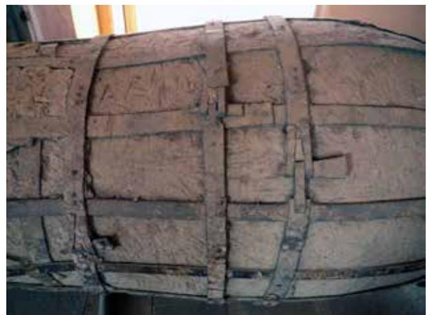
**Detail of the iron reinforcing straps showing the way they were tightened around the mould using wedges to draw the ends together**
