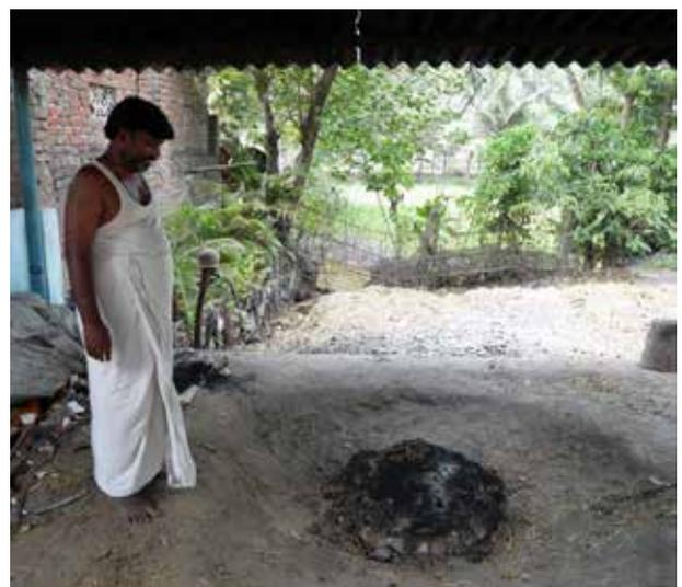
**The mould is then baked to harden it - the wax melts and runs away**
