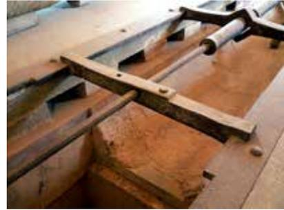
The trough in front of the 'chuck' showing the iron rails on either side and the removable cross pieces that can be used as 'steadies'
