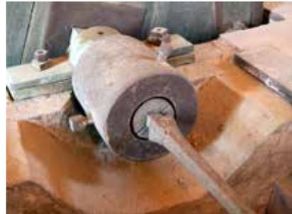
Detail of the 'chuck' with a boring bar in place
