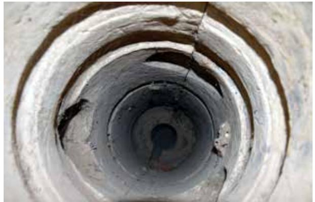
A view down the larger of the two moulds above. The join line can clearly be seen running down the length of the mould as can the trunnions at roughly 4 and 10 o'clock. The void at the top is probably decoration though this is not at all clear
