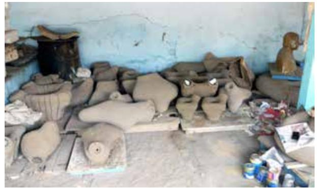
**Once the wax model is complete a one-piece mould is made. They are then left to dry for at least a week and often longer**
