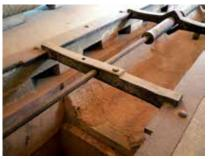
The trough in front of the 'chuck' showing the iron rails on either side and the removable cross pieces that can be used as 'steadies'
