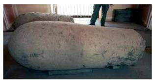
The other 2 moulds in the boring machine area both are broken and have lost their iron reinforcing straps
