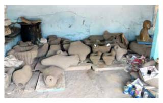
Once the wax model is complete a one-piece mould is made. They are then left to dry for at least a week and often longer
