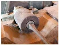
Detail of the 'chuck' with a boring bar in place
