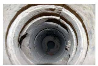
A view down the larger of the two moulds above. The join line can clearly be seen running down the length of the mould as can the trunnions at roughly 4 and 10 o'clock. The void at the top is probably decoration though this is not at all clear
