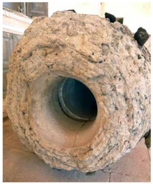
The front of the mould - the circumferential layers of the mould are clear as are the join lines at top and bottom where the two half moulds were put together. These are only visible for about 100mm showing that the mould halves were reinforced that far before being put together and the final 150mm added over the whole mould
