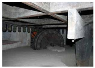
The underside of the main gear wheel showing its teeth and the second 'squirrel cage' gear wheel
