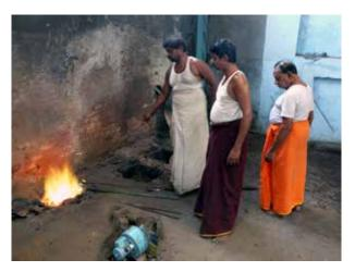
A small crucible of bronze is being heated up air is pumped into the fire by the small electric fan in the foreground
