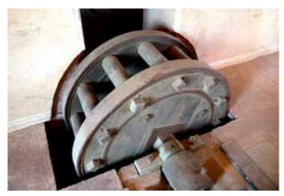
The final and fourth gear wheel - it is driven by a third gear beneath the floor which was impossible to photograph. The wall has been cut back to accommodate the wheel leading us to think that there has been some adaption or change to the original configuration. The 'chuck' to hold the boring bar is mounted directly in front. The gear, like the second and third gears, runs on copper alloy bearings, one of which can be seen here between the gear and the 'chuck'
