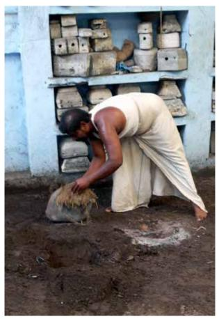
Once the mould is baked and hot and the wax has run out it is carried to the casting floor where a small depression has been made for it
