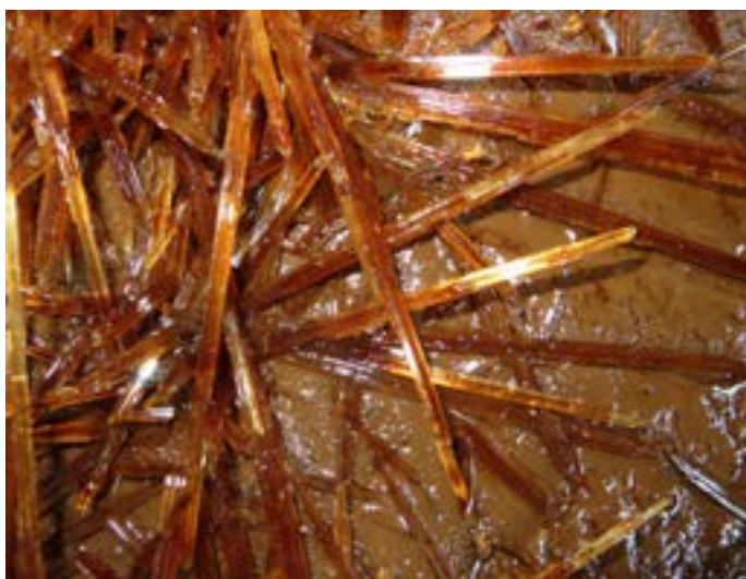
Detail of the crystals. Their long needle-like appearance is strong evidence that this is saltpetre. The contemporary record describes them as looking like ickles - icicles. The brown colour comes from the liquid.
