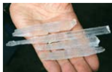
Saltpetre produced in India by a similar process showing their long needle-like crystal structure
