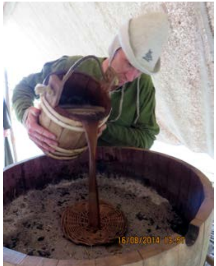
Pouring the concentrated leachate onto the bed of ashes.
