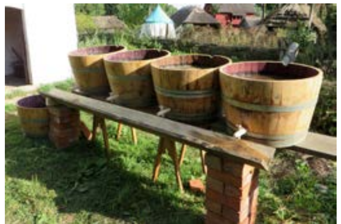
Four tubs were filled in the same way and set up on a table with a drain in front and a collecting tub at one end.
