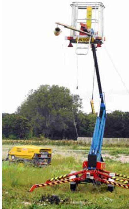
**The rig used to drop the fire pots**
