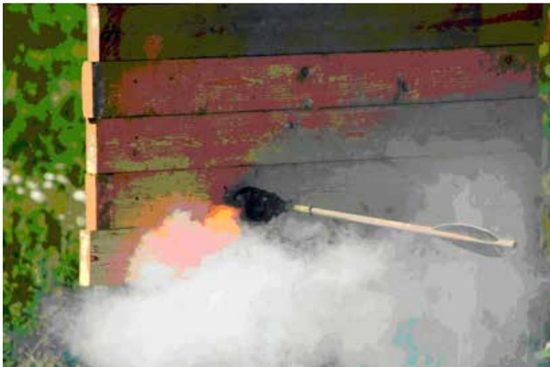
**The flame from the burning incendiary was directed towards the target by the hard coating around the arrow**
