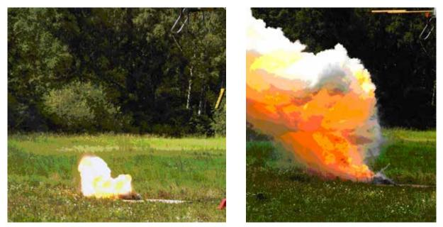
When the fire pot hits the ground it burst into flame but this only lasted for a few seconds
