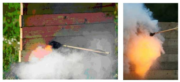
The flame from the burning incendiary was directed towards the target by the hard coating around the arrow
