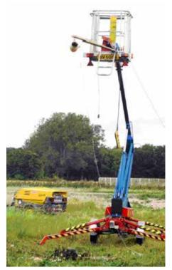
The rig used to drop the fire pots
