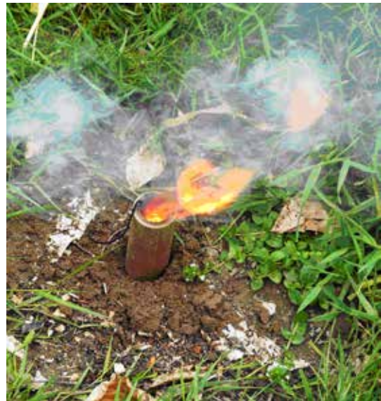
A test with the coarse powder showing that it burns slowly
