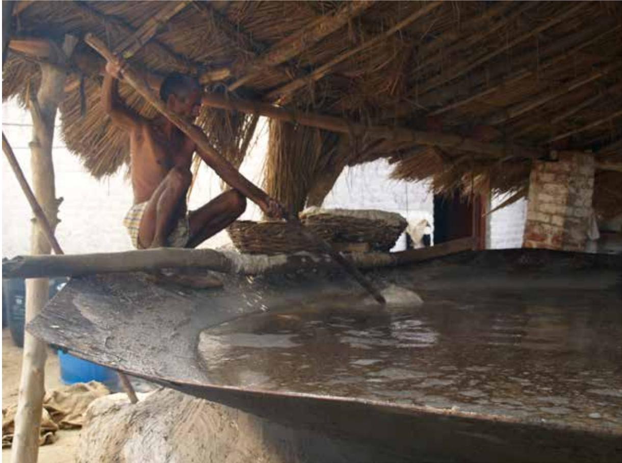
**Figure 20. Removing the salt and impurities with a large scoop**
