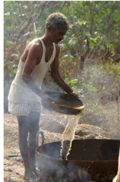
Figure 17. Pouring the saltpetre liquor into the pan
