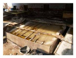
Figure 5. The settling tank with bamboo lattice on top
