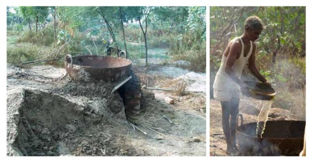
Figure 16. The pan for produing the crude saltpetre
