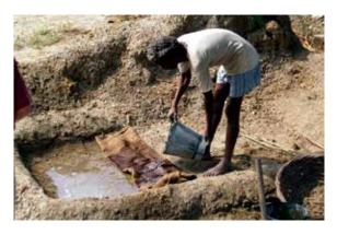
Figure 14. Pouring water over the saltpetre soil
