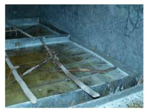
Figure 25. A precipitation tank with a lattice of bamboo on the surface of the liquid
