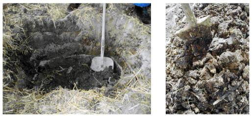
Figure 2. Left - digging out the nitre bed showing the layers of chicken shit and lime. Right – a close up of the material from the nitre bed
