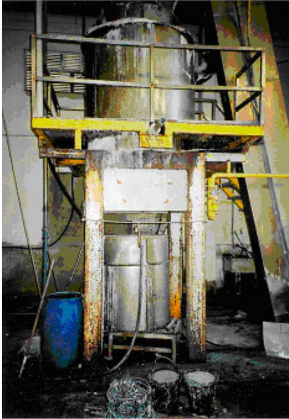
Figure 12 The iron reaction vessel
