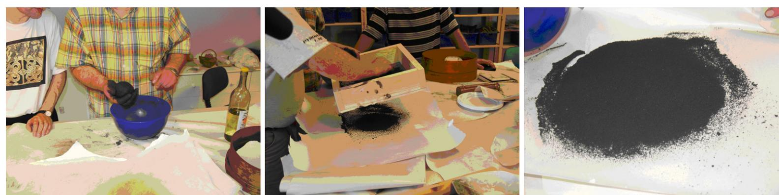
Figure 5 Left, the wetted powder prior to being pushed through the sieve (centre). Right, the resultant powder
